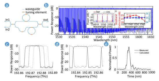
Fig. 1. (a) Chip topology; (b) Full C-band response (Insets: *i*. power response of bar and cross; *ii*. FSR and stop-band extinction); (c) demonstration of tuning; (d) demonstration of swapping; (e) Power envelope of the impulse response of the circuit.
