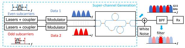
Fig. 2. Experimental setup of N-WDM generation using RAMZI Nyquist interleaver; CMZM: complex I/Q modulator.
